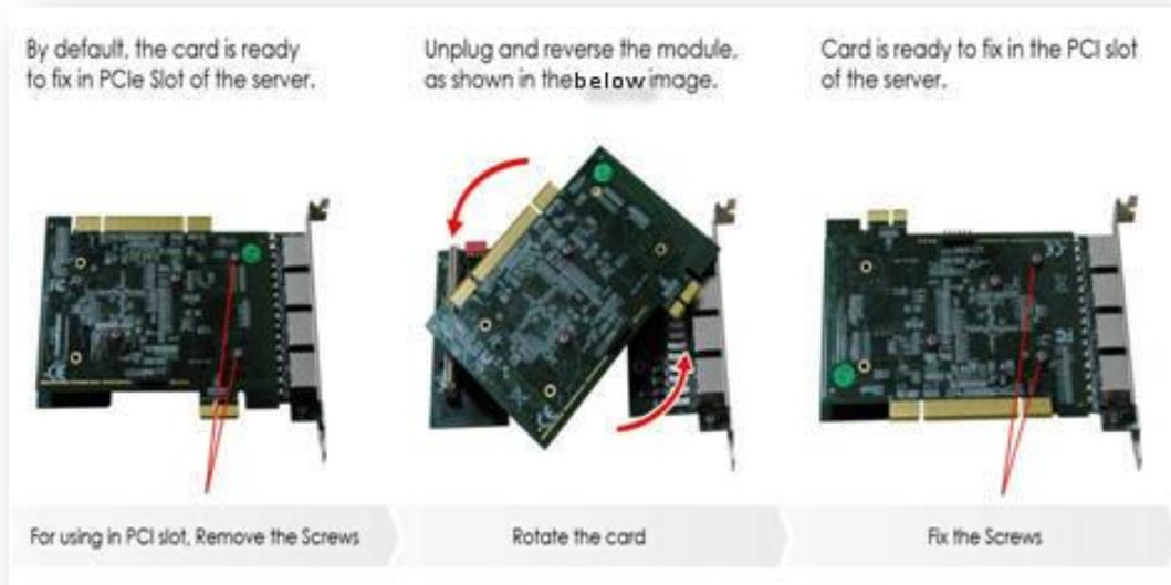
Figure 1: Customization of 2<sup>nd</sup> Generation PRI Card
