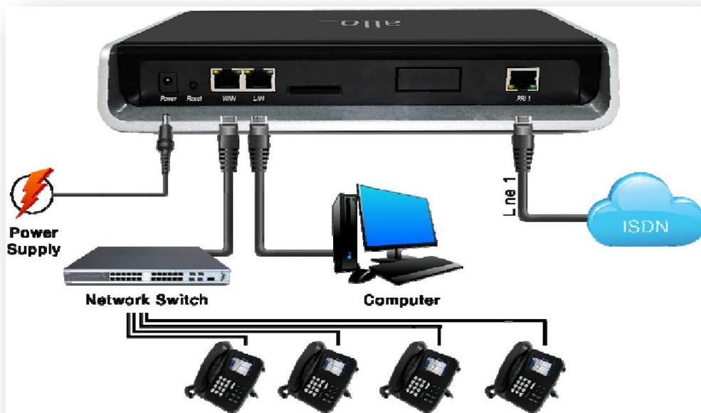
Figure 1: Initial Setup
