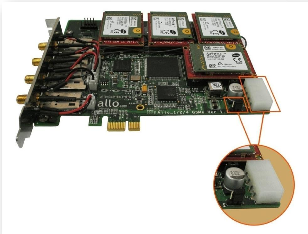
Figure 2: Power selection in Jumper Settings
