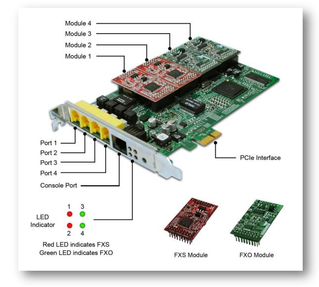
Figure 1: Hardware Setup
